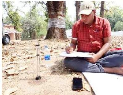
Measurement of unsaturated soil hydraulic conductivity using mini disk infiltrometer
