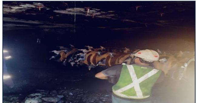
Inspection of Dust suppression measures undertaken at the source end (underground) of Padmavathi khani UG Mines, SCCL Telangana
